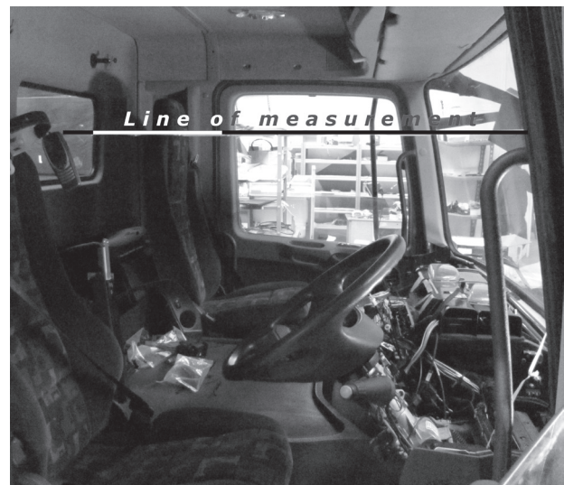
Photo 1. The setup of the exposure system for line measurements inside the Mercedes Actros simulator
